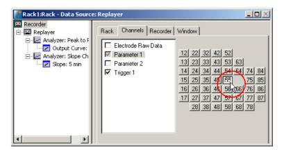
3. You can now either select all channels by clicking the check box next to the data stream name, or you can pick single channels by clicking the corresponding buttons. For more information, please see "Channel Selection" in the MC\_Rack Features section. Only data from the selected channels will be saved to the hard disk.
