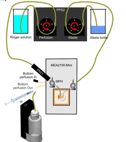
For precise and continuous suction, it is recommended to replace the syringe with the **Controlled Vacuum Pump CVP**. Set the CVP to a pressure of 15-30 mbar. The CVP will keep the negative pressure stable as long as needed. It is likely that this will result in some ACSF being sucked trough the slice (see chapter **4.2** below). It is recommended to use a valve in the tubing to the CVP, as the CVP starts working immediately when switched on.
