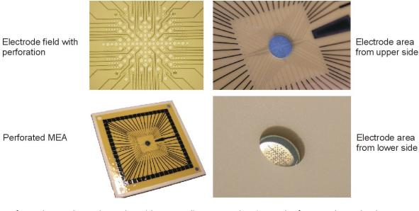
Perforated MEAs have electrodes with 30  $\mu$ m diameter and an internal reference electrode, they are available with 100  $\mu$ m a 200  $\mu$ m electrode spacing, with 60 or 120 channels.
