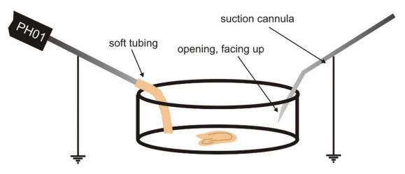
If you experience low frequency noise from the perfusion, try to optimize the suction as described above. Additionally, a **droplet isolator** can be used to interrupt the fluid flow between pump and recording chamber. The PPS2 pump from MCS is already equipped with droplet isolators. A 10 Hz high pass filter in the software can also be used to remove low frequency fluctuations in the baseline, if the amplitude is not larger than maybe 200  $\mu$ V.
