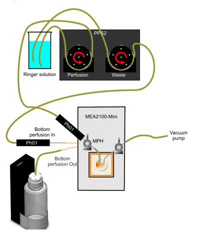
The CVP works best if the tubing to the MEA-System is short, and completely filled with ACSF. Air bubbles in the tubing are compressible, and act as pressure buffers between the pressure sensor in the bottle, and the chamber underneath the pMEA. Ideally, place the CVP as close to the setup as possible, to keep the tubing short, and put it **on the same level or above** the MEA-System. This prevents ACSF from passively flowing to the waste bottle and creating air bubbles in the tubing.
