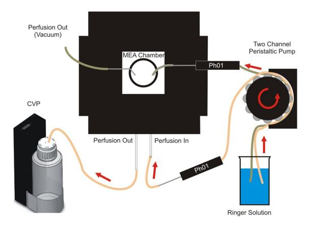
We recommend using an identical perfusion rate of 1-5 ml per minute for both perfusion cycles. Most likely, the temperature for both PH01 will have to be set a bit higher than the desired chamber temperature. Determine the **temperature offset** between PH01 and chamber with a thermometer and adjust the set value on the TC02 accordingly.
