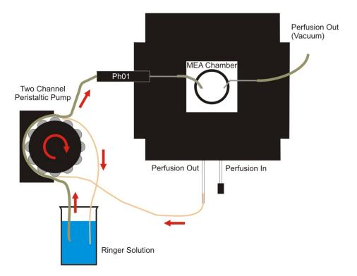
An easier and more flexible solution is to work with the **PPS2**, in combination with a vacuum pump. In that case, any flow rate can be adjusted independently for both perfusion channels without the need for specific tubing. The flow rate for the upper perfusion and the volume perfused through the slice can be varied just by setting the respective flow rates in the pump control.
