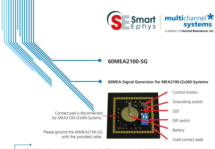
60MEA2100-Signal Generator is a very convenient tool for MEA-System users. Use the 60MEA2100-SG instead of setting up a complete experiment for training, controlling, and troubleshooting purposes.
