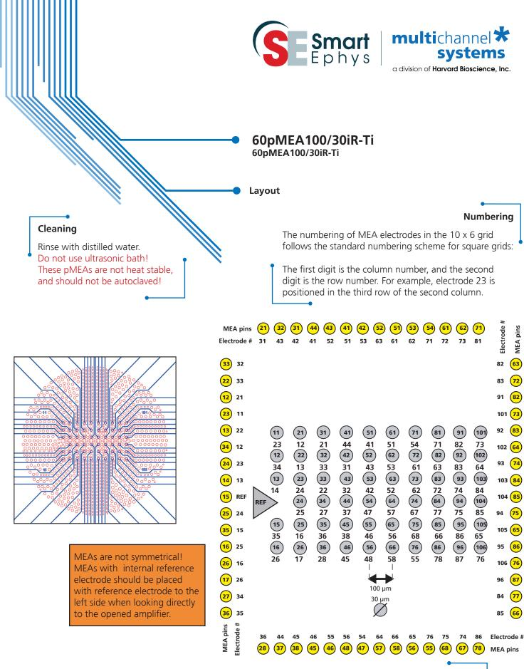
The specified MEA pin numbers (1 dim. or 2 dim.) are the channel numbers that are used in the data acquisition program, when using the 1 dimensional layout or the 2 dimensional layout (or Configuration) in the "Data Source Setup". The electrode 14 is missing in MEAs with internal reference electrode. It is replaced by a big internal reference electrode, connected to pin 15 of the amplifier.
