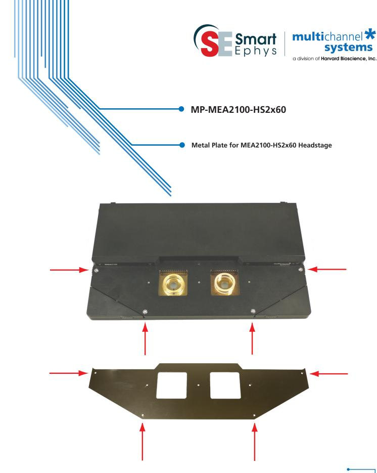
For installing the metal plate, please remove the four designated screws on the headstage of the MEA2100 device and keep the screws for reusing them later. Attach the steel plate onto the headstage and fix the plate with the four screws.
