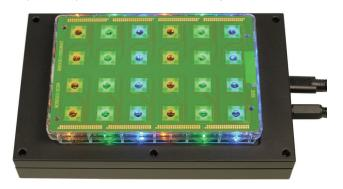
The MW24-opto-stim fits upside down on top of a 24-well plate, with or without lid. The device may be used in combination with the Multiwell-MEA-System, or as stand-alone solution.
