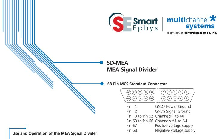
The MEA Signal Divider is used for picking single channels from the MEA amplifier. It is connected to the MEA1060 amplifier and to the MC\_Card or to an USB-ME-System with 68-pin MCS high grade cables. The pin layout follows the MEA layout. It does not matter to which socket the input or the output is connected.
