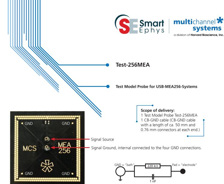
For the intention to check the noise level of an USB-MEA256-System without external signals, please connect "Signal Source" and "Signal Ground" sockets with a CB-GND cable for a short circuit. All 252 recording electrodes are internally connected to the resitor-capacitor pair.
