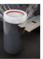
The TOOL now becomes a guide so that the excess membrane sheet can be cut away with a sharp razor blade or scalpel. Always leave 2-4mm of foil beyond the O-ring for a secure fit. Be sure to use a sharp blade so that the foil is completely cut. Pulling on the foil can cause ripples across the membrane.
