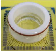
O-ring into the inner groove until it is worked in all the way around.
