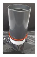
Place O-ring (#21) over the end of the insertion tool on the shallow cut side
