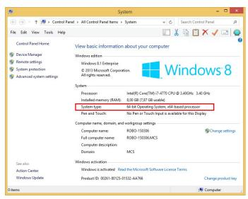
Open the "System" dialog from the Windows "Control Panel" and check the "System type".
