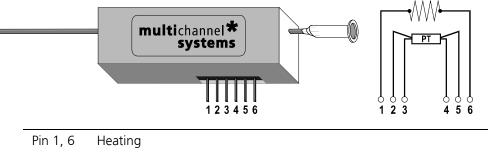
Pin 2, 5 Temperature sensor power supply
