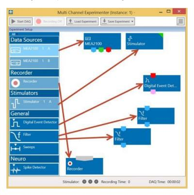
It is also easy to connect the instruments: Please click onto one of the symbols on the lower part of an instrument button to connect this output port via drag and drop with the input port (symbol on the upper side) of the target instrument. Please read the next chapter.
