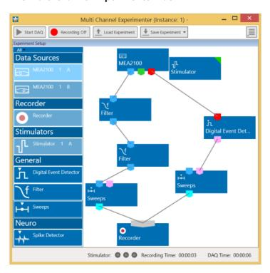
Move as many instruments as you need via drag and drop into the "Experiment Setup" window. It is possible to use the virtual tools more than one time.
